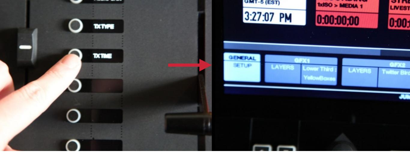
You can return to the main **General Setup** menu display by pressing the currently activated setup menu's **menu button**.
