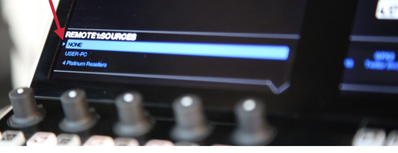
The left arrow indicates which source is currently being seen in the remote camera module.
