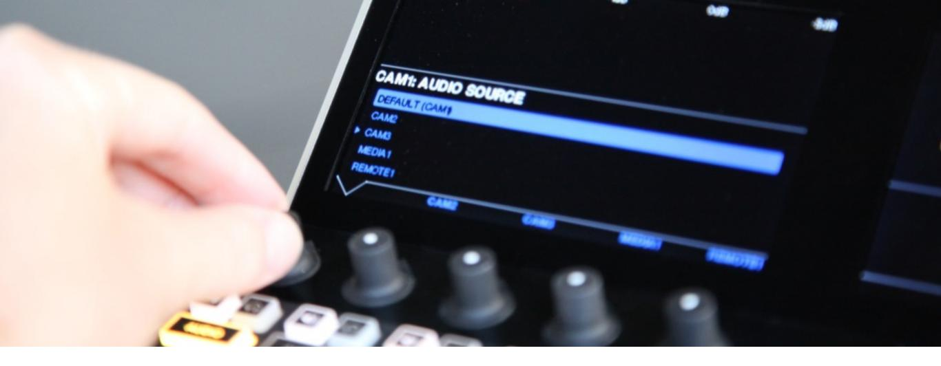
You can revert audio linking by going back to the audio source menu for that video source and scrolling up to the default setting of using its own audio.
