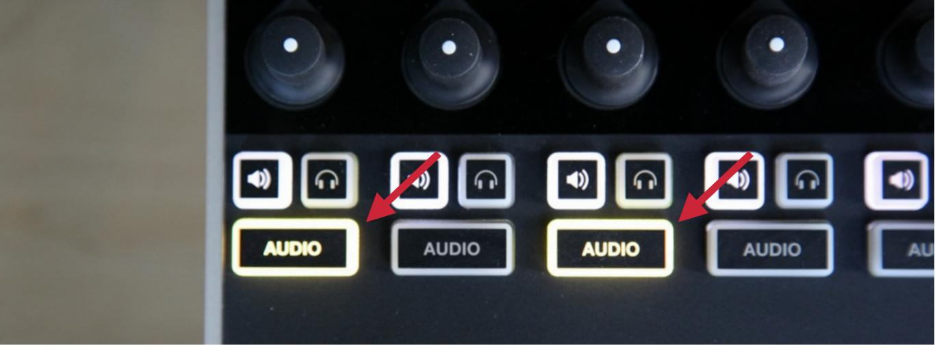
When either source is in Program, both audio control buttons will light up, indicating that both sources have the same audio.
