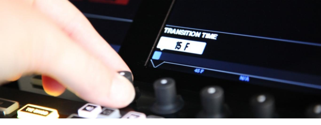
Just as with transition type, the main mix and the three graphics overlay channels can have independently set transition times. ('**Cut**' cannot have a set time.)
