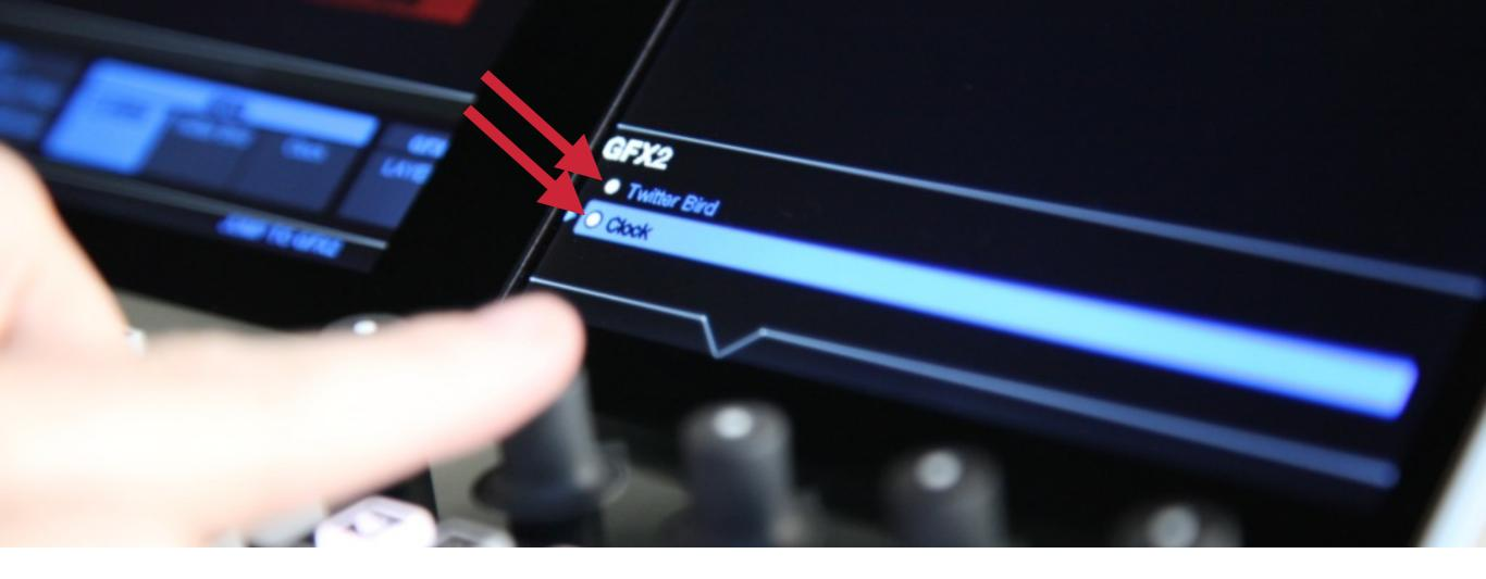
The **white dots** indicate a layer that will be visible when that graphics overlay channel is in Preview or pushed to Program.
