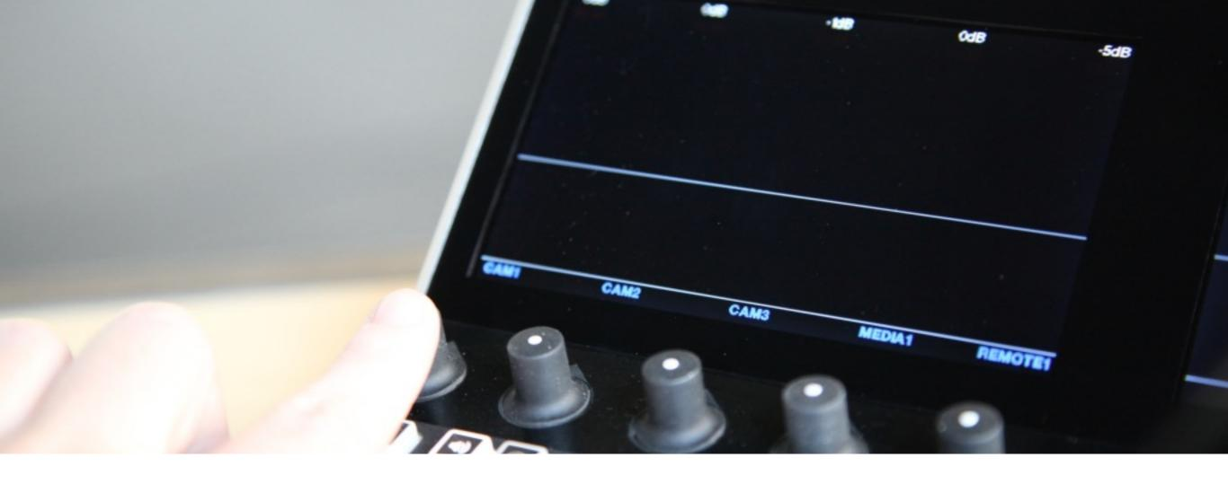
You can change any of these input sources' track assignments directly from Studio Surface. Press down the knob corresponding to the source you want to change.
