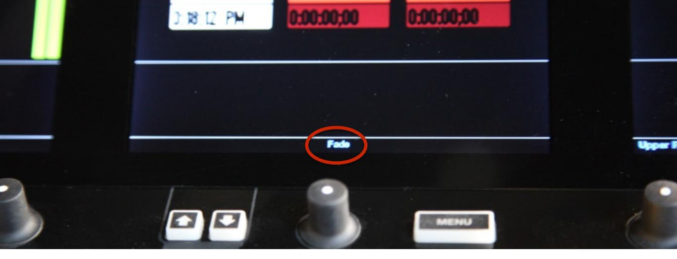
You should notice in the bottom of the middle monitor, there is a name of a type of transition above the control knob.
