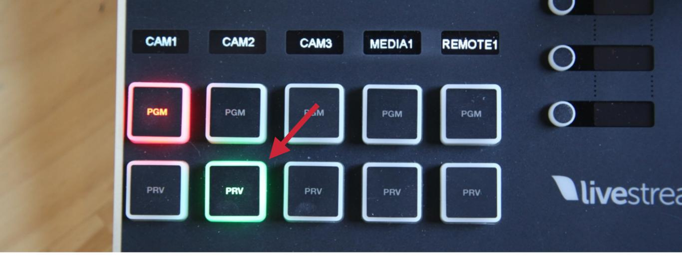
To put a source into Preview, press the green '**PRV**' on the track that corresponds to that input source.
