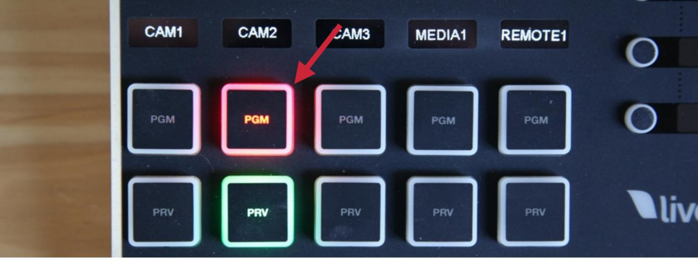
You can also directly put a source into Program without previewing it. To do so, press the '**PGM**' button that corresponds to it.
