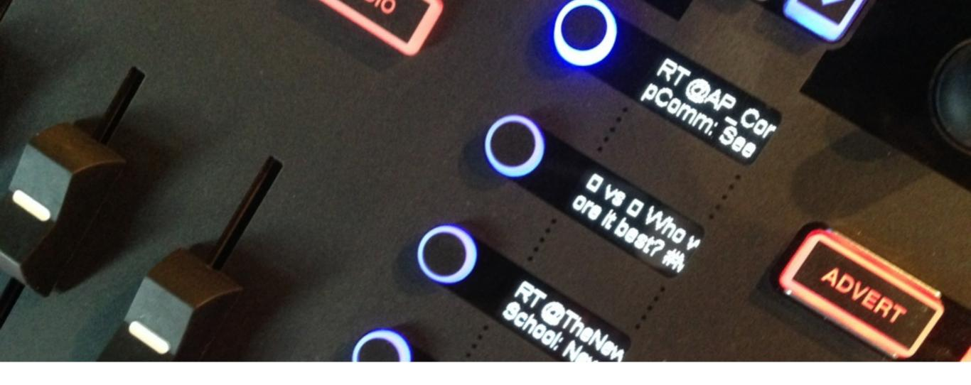
After selecting a layer, the **menu buttons** will display the rows of data available in that layer, such as a manually built row, data from a spreadsheet, or tweets.
