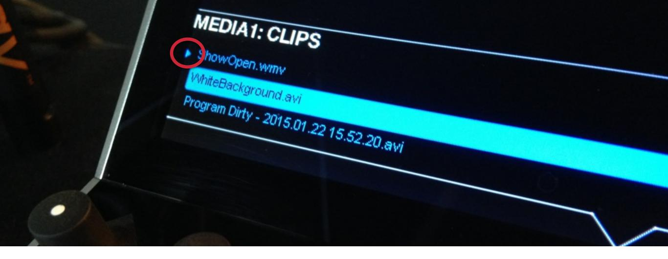
The arrow on the left indicates which clip is currently queued up. Turn and press in the knob to select a different clip.
