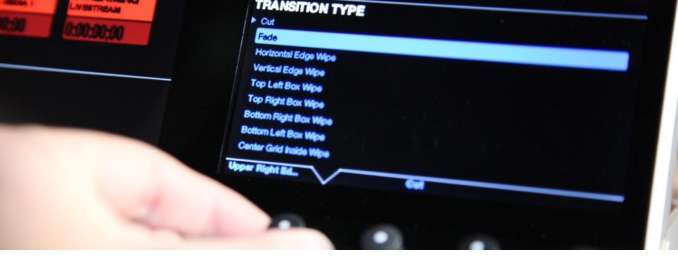
On the right monitor, you will have the option to select different transitions for your three graphics overlay channels. Press and turn the corresponding knobs to do this.
