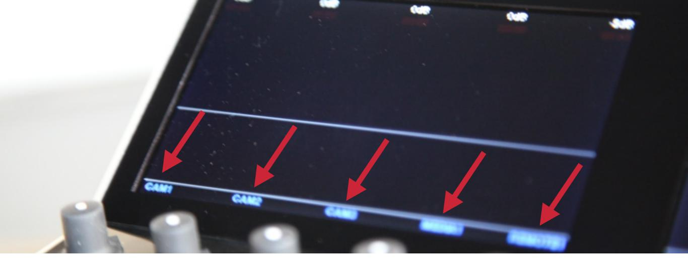
On the left monitor, you should notice that the names of your 5 input sources appear on the bottom of the screen.
