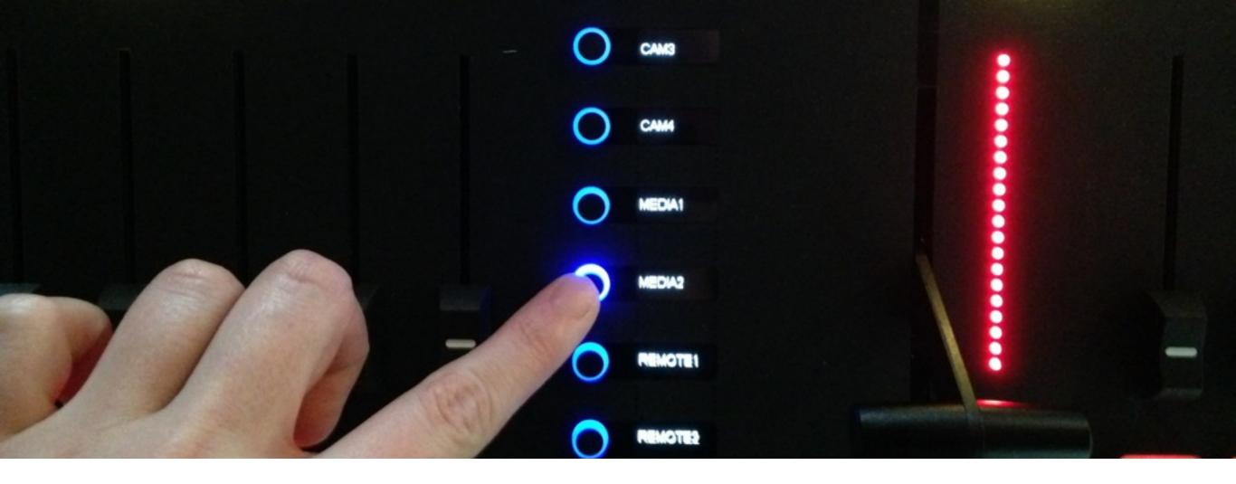
Press any of these buttons to hot change the source that is being used for that AUX. The change will immediately be shown in any graphic or output using that AUX.
