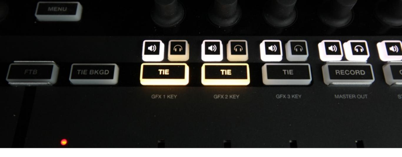
If only the GFX 1 and GFX 2 '**TIE**' buttons are lit and both sources are in Preview, then both overlays will switch into Program when transitioning. The video will not change.
