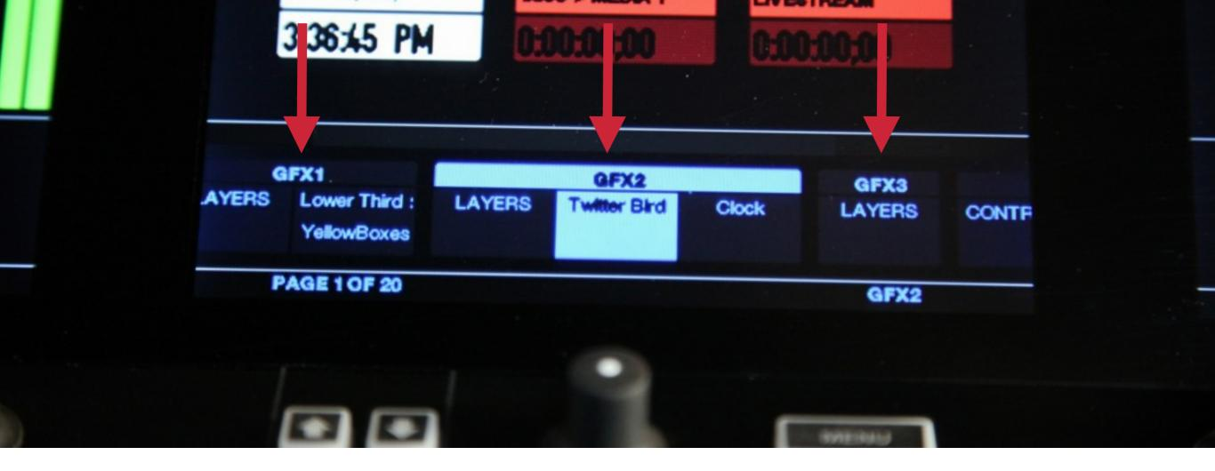
The layers menu and the ability to change data are available for all 3 graphics overlay channels. Use the knob to scroll to the other channels.
