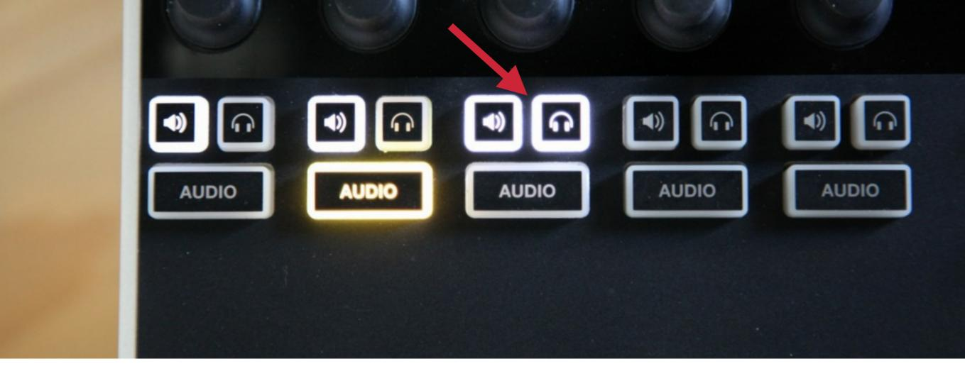
You can use these buttons to isolate each audio source before going live and adjust their levels as needed.
