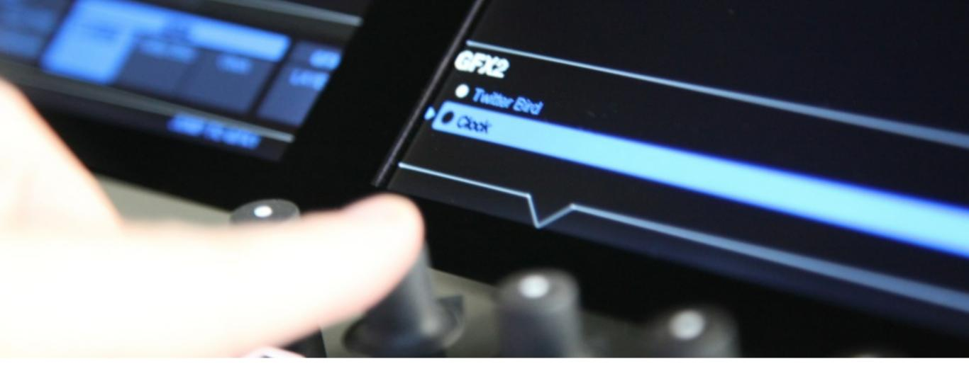
When a layer is selected, press in the knob to switch the layer's visibility. More than one layer can be visible at a time.
