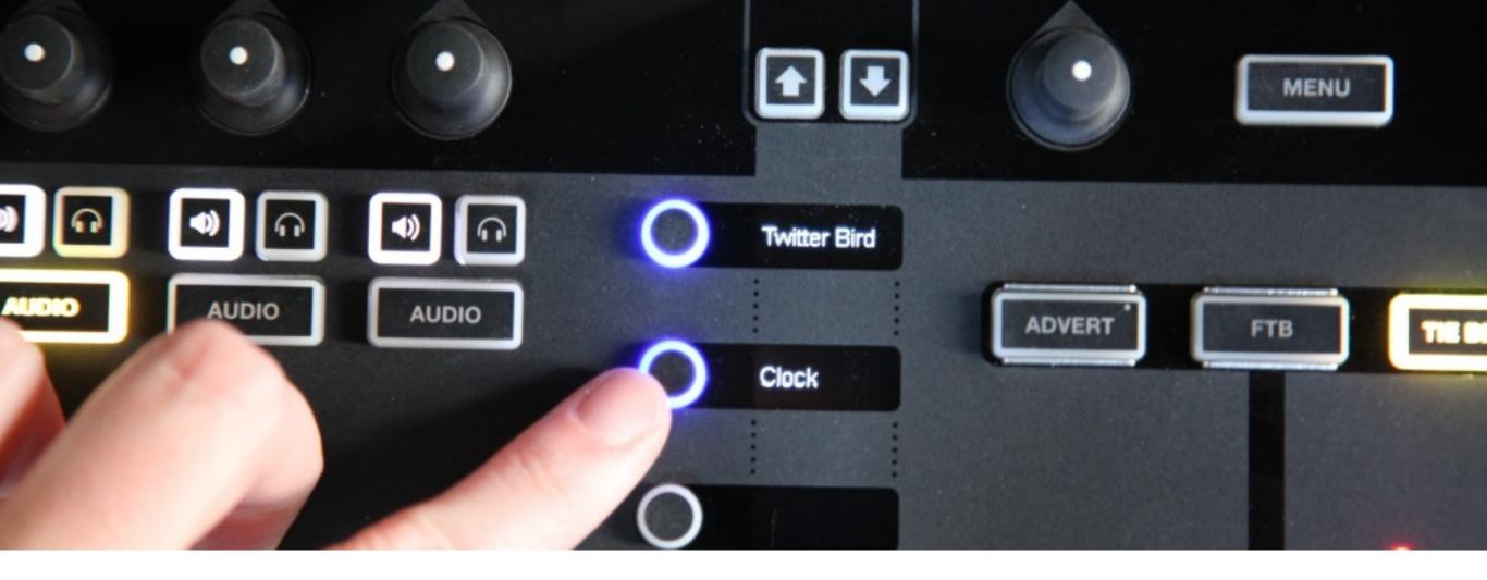
The buttons that are lit up indicate which layers in that GFX channel are visible when in Preview or Program. Pressing the respective button will turn visibility on or off.
