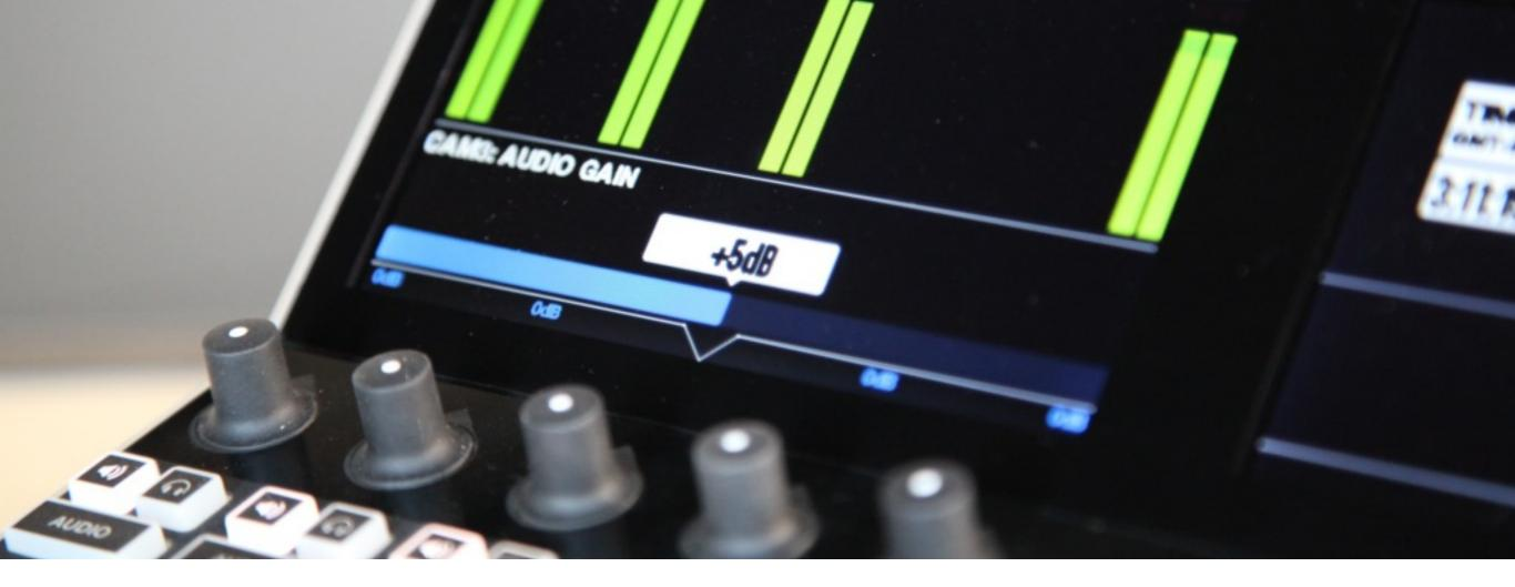
A **gain meter** will immediately appear as you adjust the audio source's gain level. Press down the knob when you have reached the desired level.
