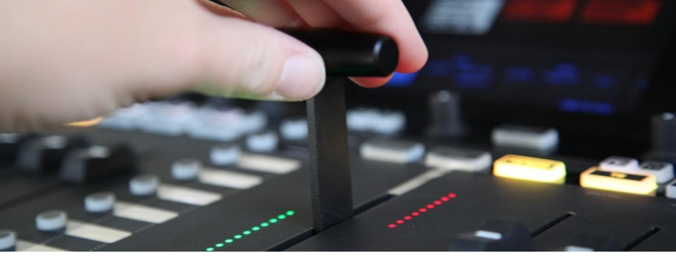
Another way to use that transition is to manually switch your sources using the **T Bar** on the Studio Surface. This allows you to control the transition's speed.
