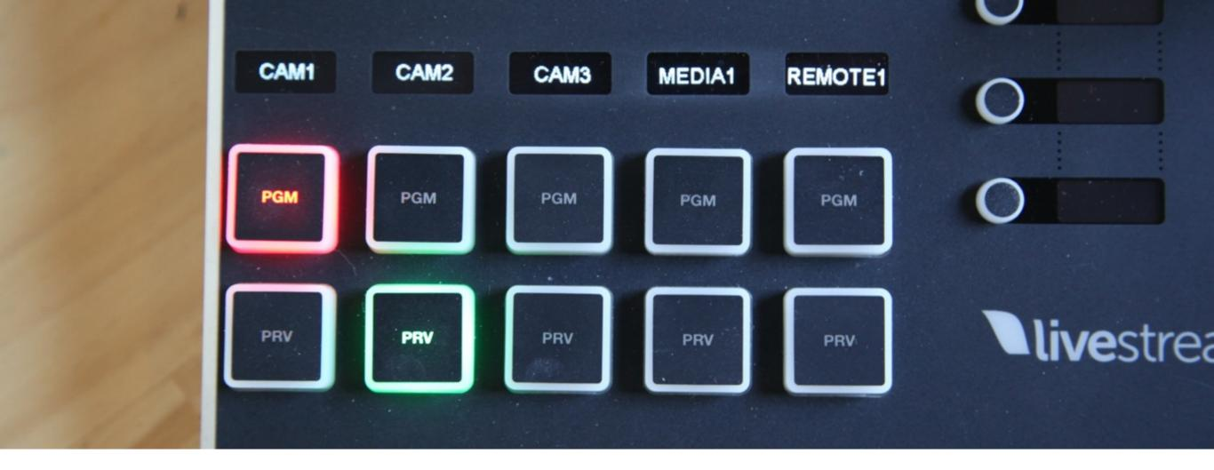
The bottom left corner has the Preview (**PRV**) and Program (**PGM**) controls for 5 assigned input sources.
