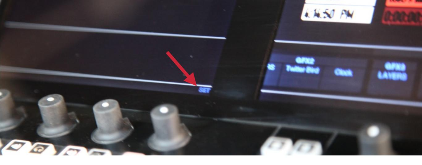
The track that the camera is assigned to should start blinking '**SET**' at the bottom of the monitor. Press in the corresponding knob.
