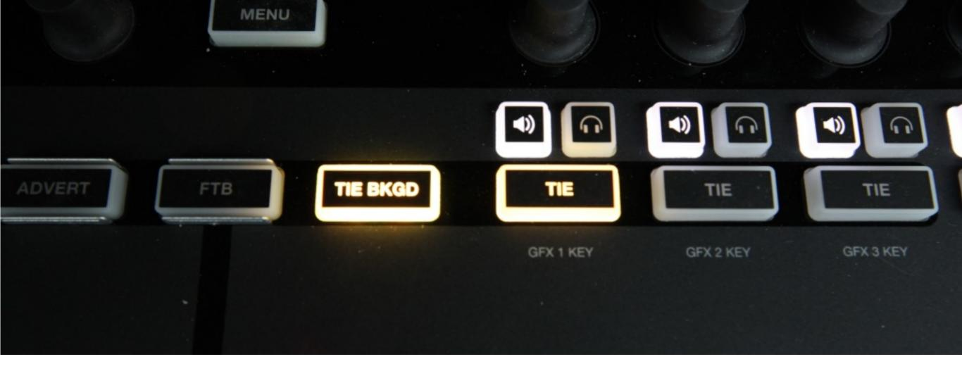
To pull a graphics overlay out of Program simultaneously with a video source, tie the background and the graphics overlay together.
