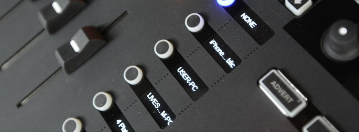
When selecting from either remote camera module, the **menu buttons** will display each remote source that is available to you in Livestream Studio.
