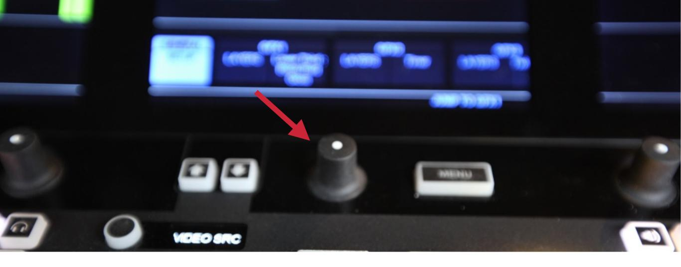
You can navigate to each menu using the black knob in front of the monitor. Start with the **General Setup** menu.
