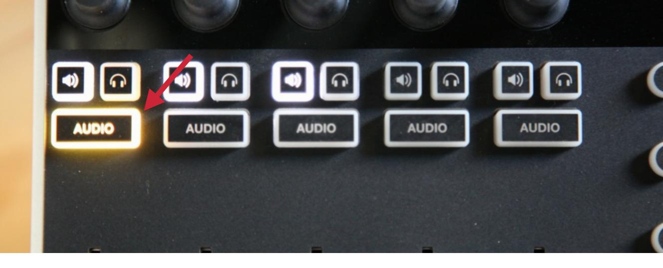
When switching between your video sources, you may notice different audio controls on the left lighting up and turning off during transitions.
