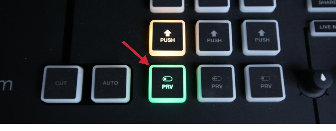
Press the '**PRV**' button for the graphics overlay channel that is tied to your video source.
