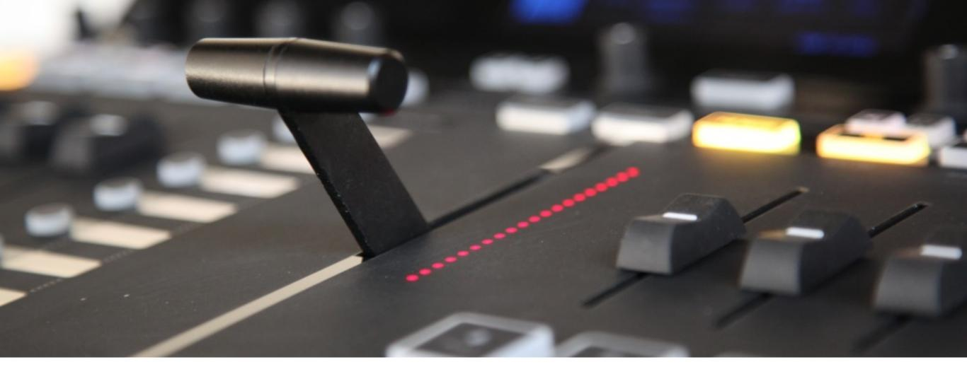
Above the '**Cut**' and '**Auto**' buttons is the **T Bar**, which allows you to do a manual transition between Preview and Program in Livestream Studio.
