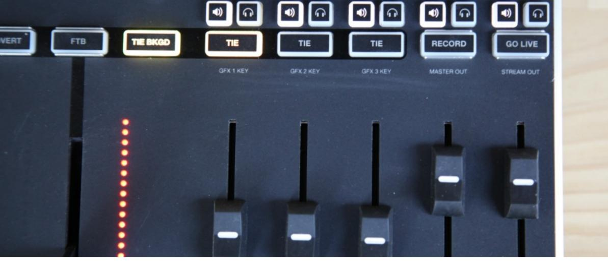
Under the right monitor are controls that adjust the audio levels for the corresponding graphics overlays, Program record, and Program stream.
