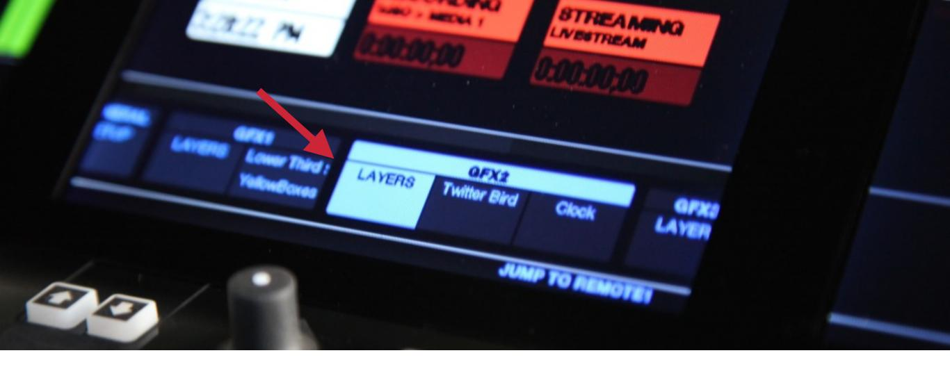
One type of assignment you can set is for viewing all the layers within that graphics channel. First, select the layers menu within that channel.
