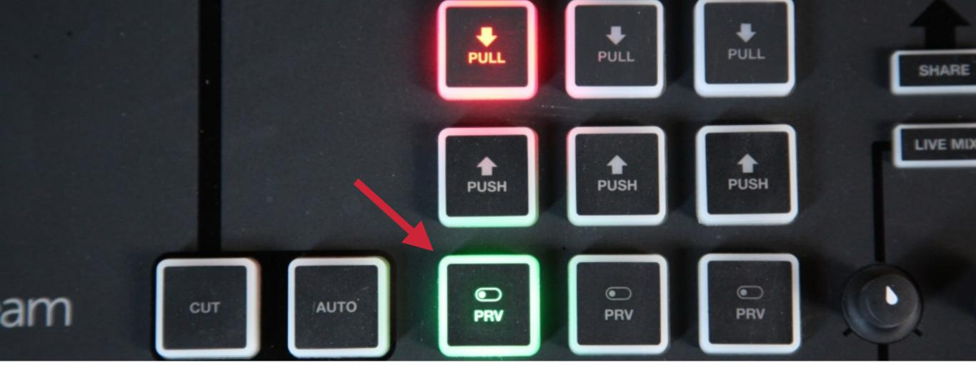
Next, you will need to remove the graphics overlay from Preview. This will tell the transition controls that the graphic is not being shown on the next switch.
