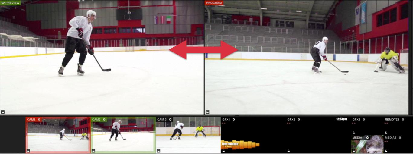
A typical multi-camera production involves putting a source into Preview and then switching it with the source in Program using a transition control.
