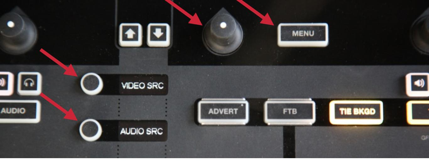
The controls for these menus include the knob below the monitor and the **menu buttons** running down the center of the Studio Surface.
